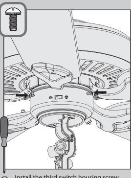
Install the third switch housing screw.
